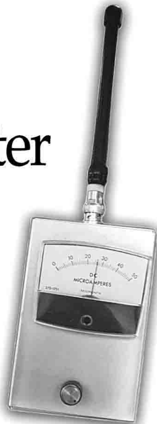
The RF Signal Strength meter responding to my Kenwood TH-26AT transmitting on 147.900 MHz with 1 W, 2 feet away from the meter. The sensitivity control is set at mid range.
